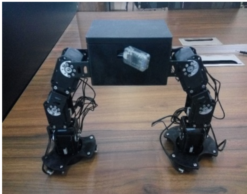
Figure 2. Practicality picture of the biomimetic adherent inchworm-like robot 图 2. 仿生粘附式尺蠖机器人实物图
