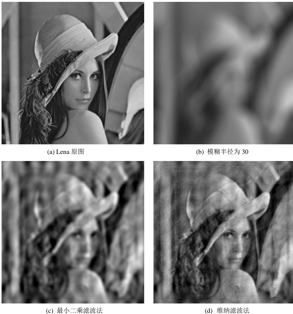
Figure 2. The comparison of Weiner and least square filter 图 2. 维纳滤波与最小二乘滤波复原方法对比
