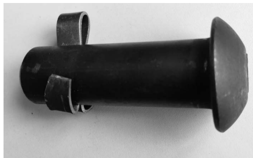
Figure 1. The relationship between the flat cotter pin and the brake pin 图 1. 扁开尾销与制动圆销的相对关系
