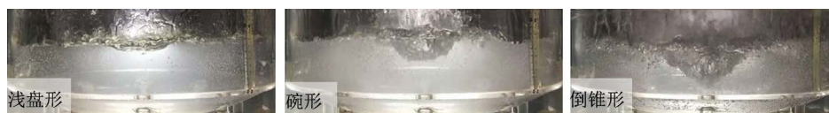
Figure 2. Typical shape of the impacting pit 图 2. 典型的冲击坑形状
