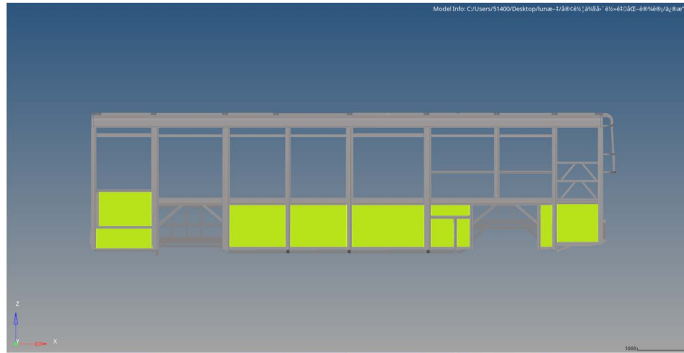
Figure 4. Topology optimization area on the left 图 4. 左侧拓扑优化区域
