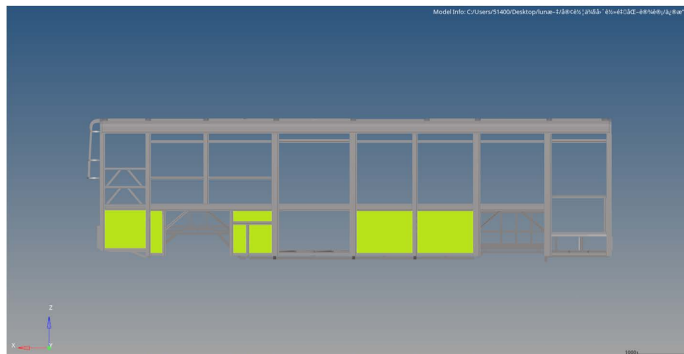
Figure 5. Topology optimization area on the right 图 5. 右侧拓扑优化区域
