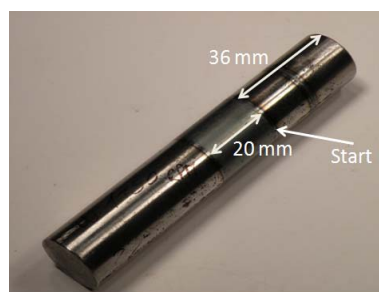
Figure 13. A wider cylindrical hardened surface obtained by VS technique 图 13. 利用可见光斑法得到的更广泛的圆柱硬化表面
