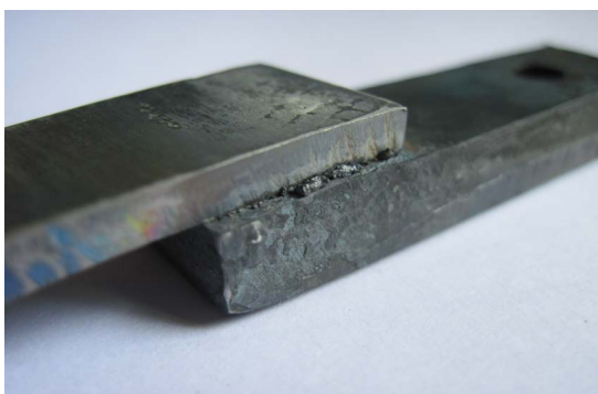
Figure 2. Brazing sample of TA2/Zr-Ti-Ni-Cu/Q235 图2. TA2/Zr-Ti-Ni-Cu/Q235 高频钎接头试样
