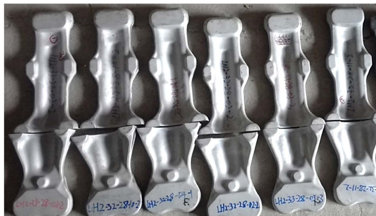
Figure 1. Hand forging of SiC/2009Al matrix composites
