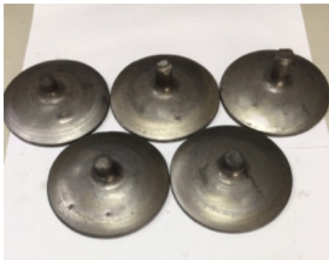
Figure 4. Ta-W alloy EFP liners after forging 图 4. 钽钨合金 EFP 药型罩锻造毛坯
