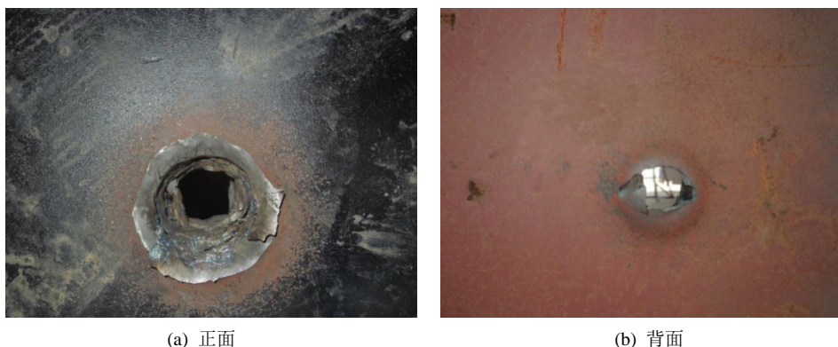
Figure 7. Target damage of EFP liner 图 7. 战斗部着靶情况
