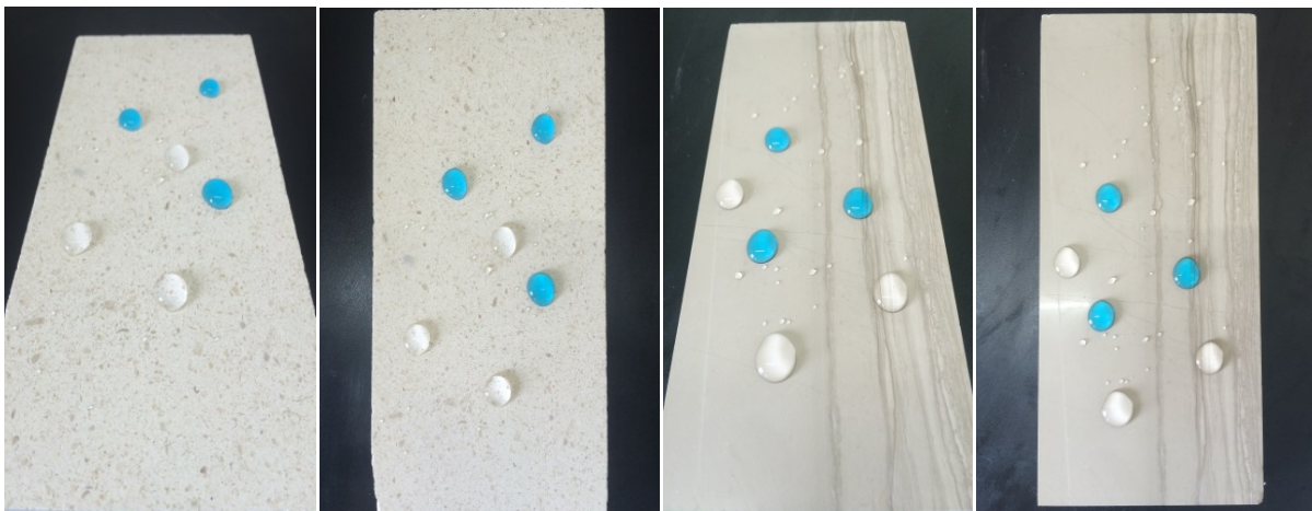
Figure 4. Digital photos of superhydrophobic coating after exposing to outdoor for 4 months
