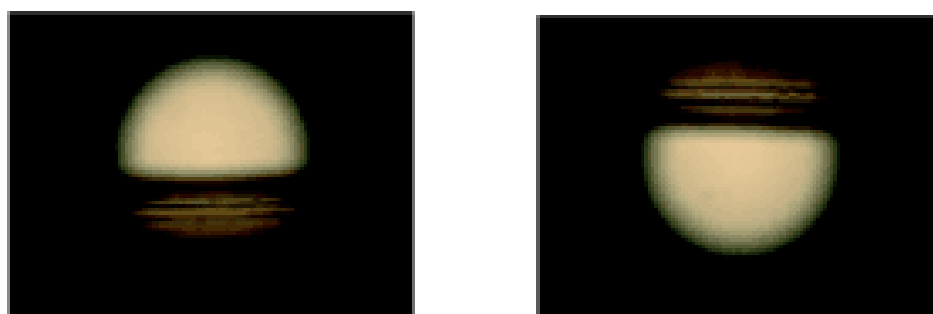
Figure 4. A group of symmetrical focal spots (the system magnification is 10)
