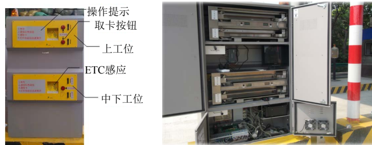
Figure 4. 3 locations' card machine (left) and the card slot (right) 图 4. 上中下工位发卡机(左图)及卡槽(右图)
