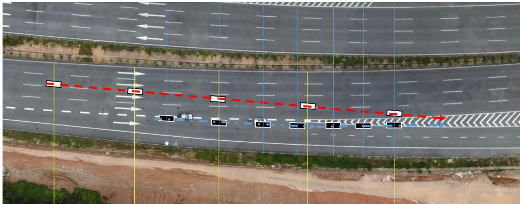
Figure 4. Two vehicle running track before the incident 图 4. 事发前两车行驶轨迹
