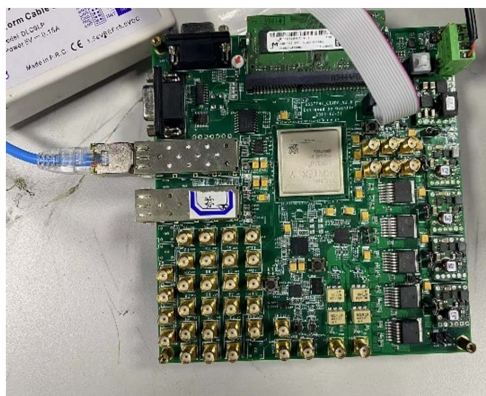
Figure 6. Diagram of the central control board card 图 6. 中控板卡实物图
