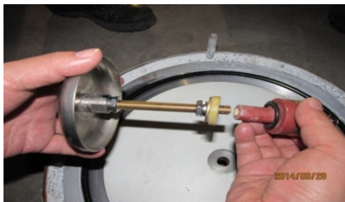
Figure 3. Diagram of the fracture of the built-in probe of the charged display device 图 3. 带电显示装置内置探头断裂示意图
