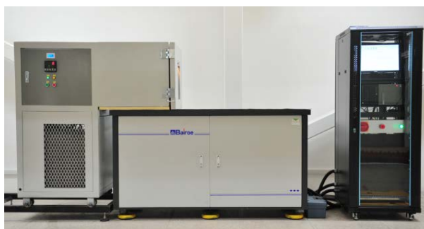
Figure 1. FPL-600 transverse vibration test system
