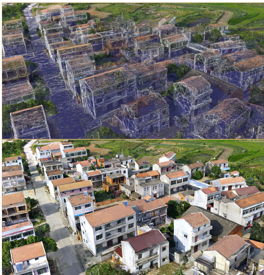
Figure 2. Irregular triangular meshes and 3D texture mapping 图 2. 不规则三角网和三维纹理映射
