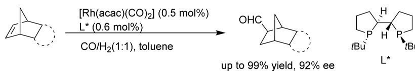
Figure 25. Rh-catalyzed asymmetric hydroformylation of norbornene derivatives
