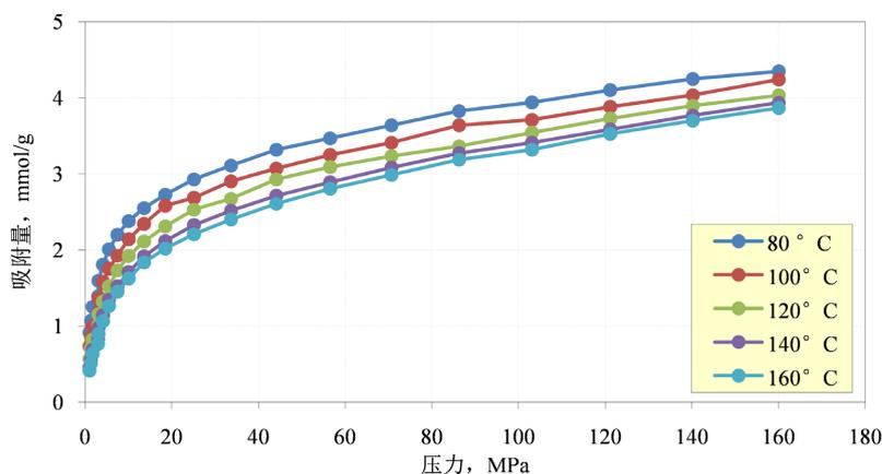
Figure 1. Isothermal adsorption curves of deep shale gas
