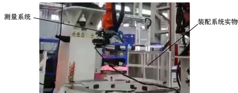
Figure 2. Physical measurement and assembly systems
