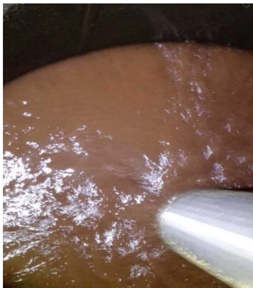
Figure 1. Drainage diagram after regeneration (resin decomposes under the influence of high temperature)
