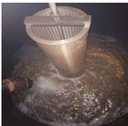
Figure 2. Drainage diagram after regeneration (resin decomposes the undecomposed state of the resin)
