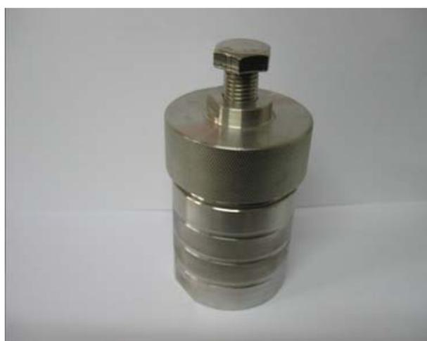
Figure 10. Autoclave for water thermal reaction in the experiment
