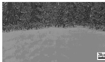
Figure 3. Section morphology of nickel plated brazing joint
