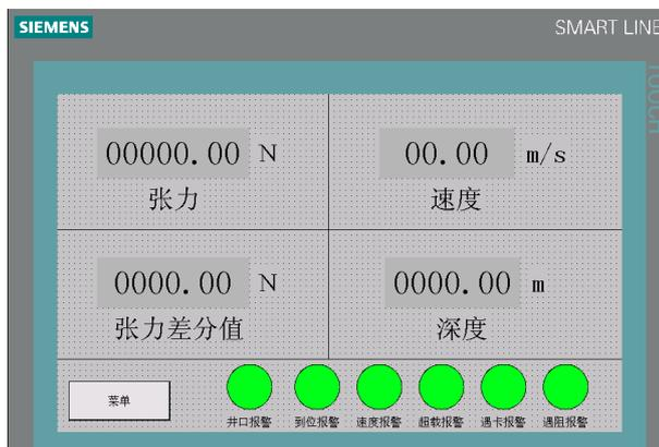
Figure 2. Winch parameters monitoring interface
