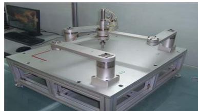
Figure 17. The experiment platform of 2-DOF redundantly actuated parallel robot
