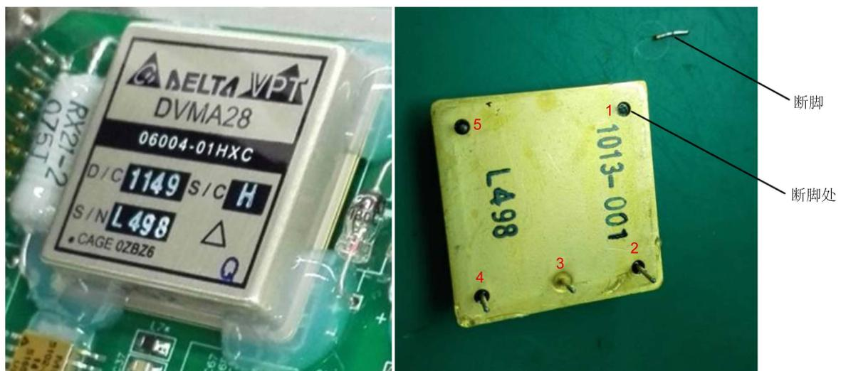
**Figure 2.** The fracture of the pin in the chip (the 1st pin)
