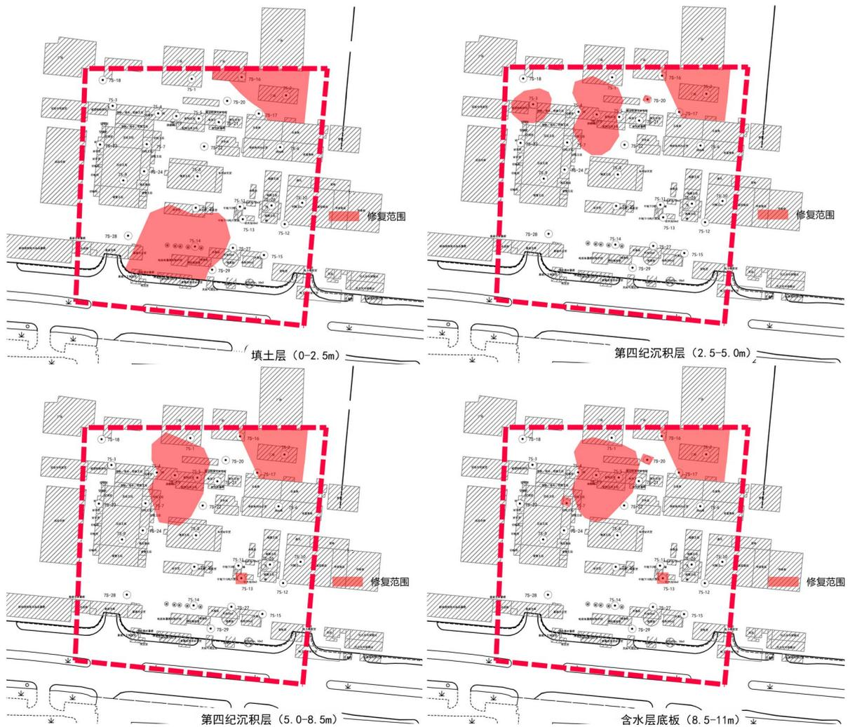
**Figure 3.** Schematic diagram of remediation scope
