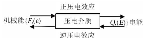
Figure 1. The reversibility of the piezoelectric effect
