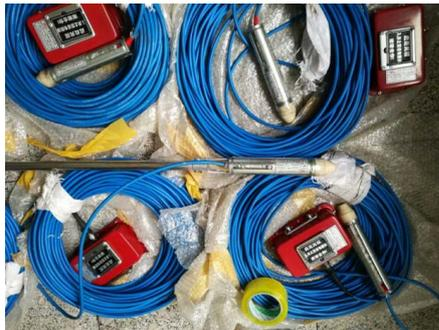
Figure 1. Mining floor stress monitoring equipment
