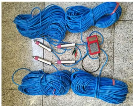
Figure 2. Mining floor osmosis, temperature monitoring equipment
