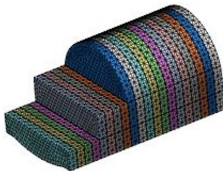
**Figure 2.** Schematic diagram of excavation step of station
