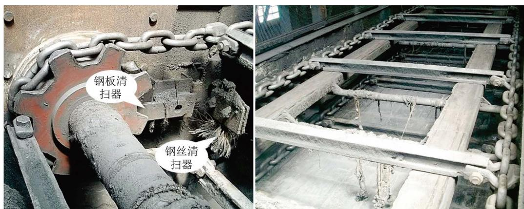
Figure 4. Internal structure of the modified scraper conveyor
