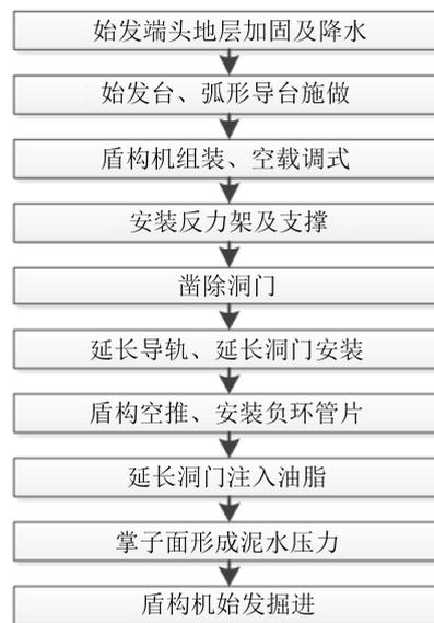
Figure 3. Shield tunnel initiation flow chart
