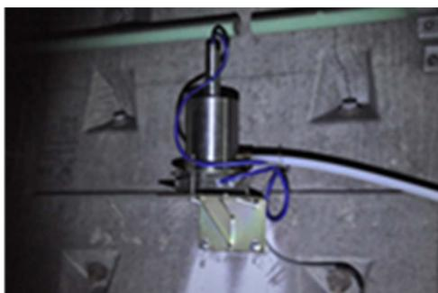
Figure 2. Hydrostatic leveling sensor on tunnel
