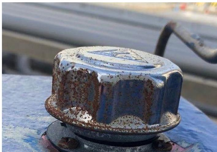
**Figure 2.** Corrosion of electro galvanizing surface
