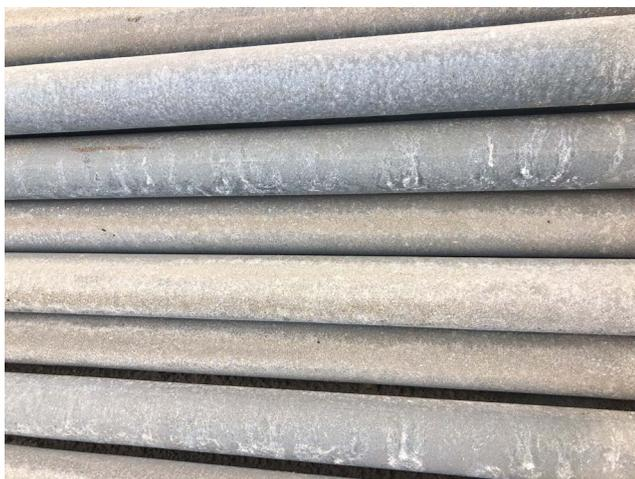
**Figure 3.** Corrosion of hot dip zinc surface
