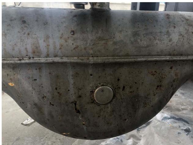
**Figure 6.** Corrosion of stainless steel 316 surface
