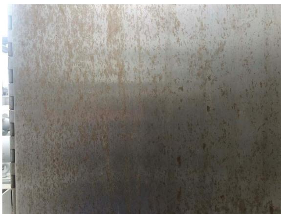
Figure 5. Corrosion of stainless steel 304 surface
