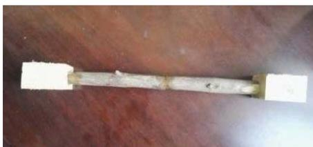
Figure 1. Small hardwood blocks installed at both ends of the sample
