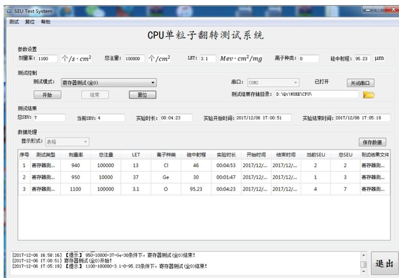
Figure 10. Register test ended with all 0
