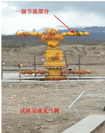
Figure 4. Schematic diagram of well tree after oil test
