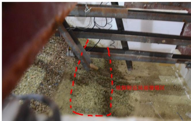
**Figure 6.** During the 0.15 g earthquake in the test, the toe of the slope collapsed locally (undisturbed slope)
