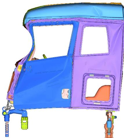
Figure 6. A pillar crash deformation
