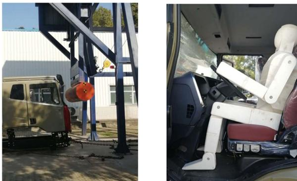
**Figure 8.** A heavy truck CAB A pillar crash test
