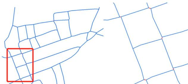
**Figure 7.** Example of a road that requires correction for starting and ending point coupling
