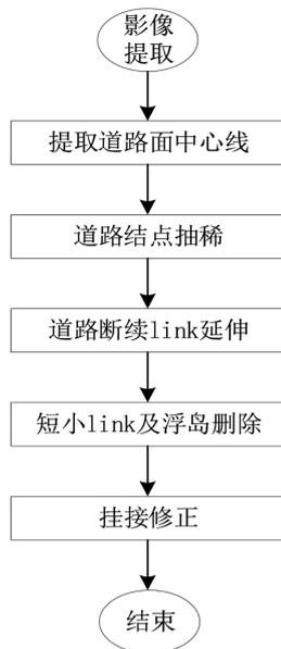
Figure 1. Road data processing process
