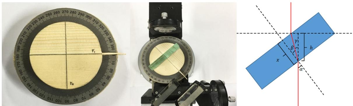
Figure 4. (a) Self-made rotatable carrier table, (b) actual placement position of glass sample, (c) light path inside and near by the sample
