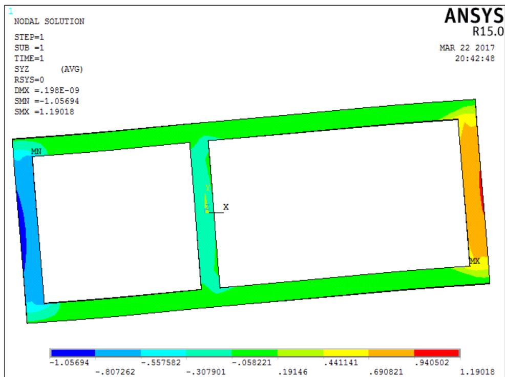
Figure 12. Contour of shear stress  $\tau_{yz}$  (unit: MPa)
