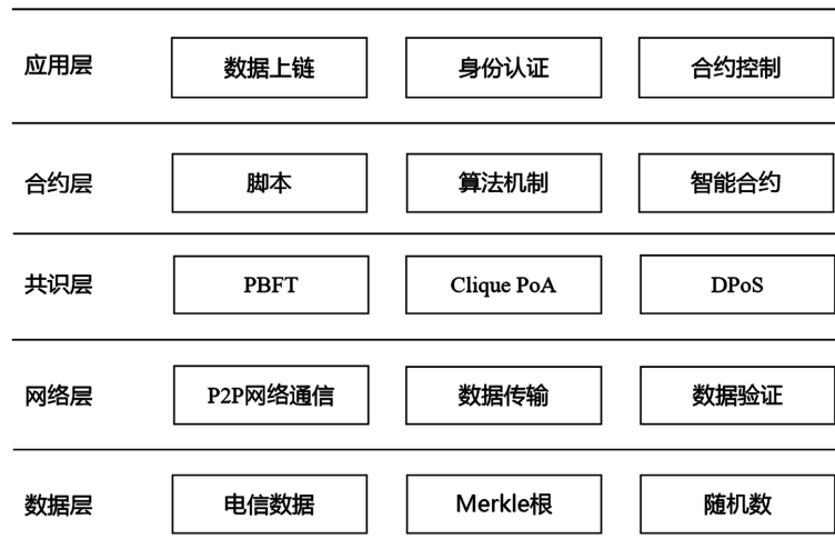
Figure 3. System underlying architecture 图 3. 系统底层架构
