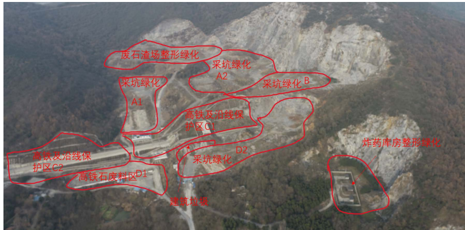
Figure 6. Zone diagram of ecological restoration in mining area 图6. 矿区生态治理修复分区图
