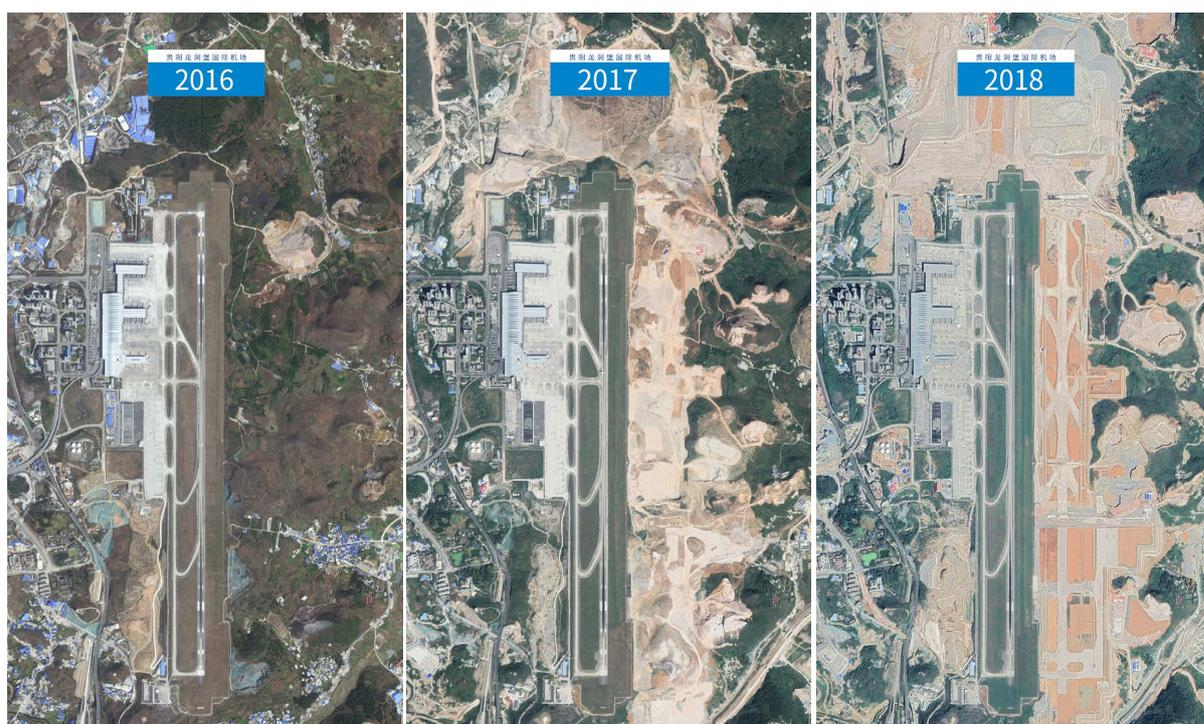
**Figure 1.** Overview of landform before and after the expansion of Guiyang Longdongbao Airport
