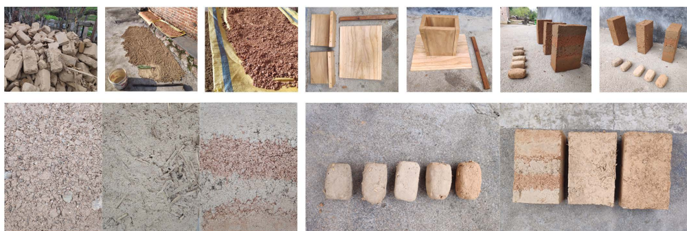
Figure 6. The process of making raw adobe bricks 图 6. 生土砖制作过程
