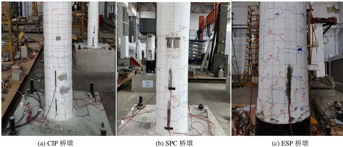
Figure 3. Bridge pier damage forms
