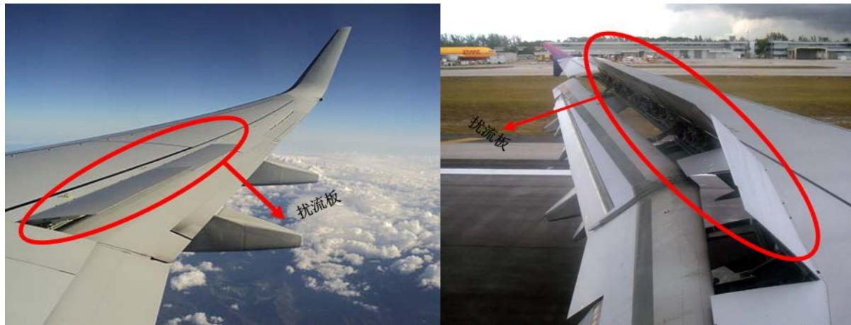
**Figure 1.** The chart of spoiler on aircraft
