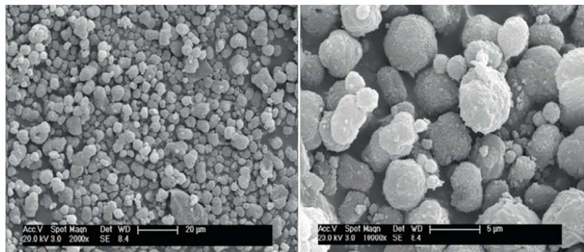
**Figure 8.** SEM of microcapsules [27]
