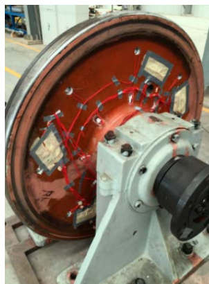
Figure 6. Installation diagram of positive pressure test instruments 图 6. 正压力测试仪器安装图
